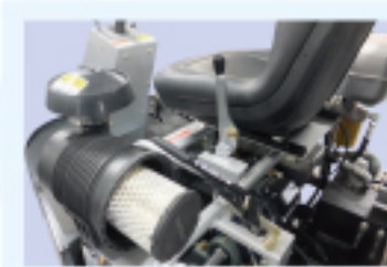
Protected the engine from sand dust by 2-layer air filter.
