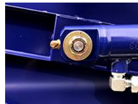
13. Front-side of the hopper lid open/close cylinders located left and right
